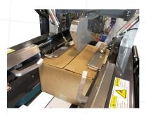
Dual side rear flap tuckers and positive folding of major flaps (Not optimal for sealing boxes filled beyond capacity)
